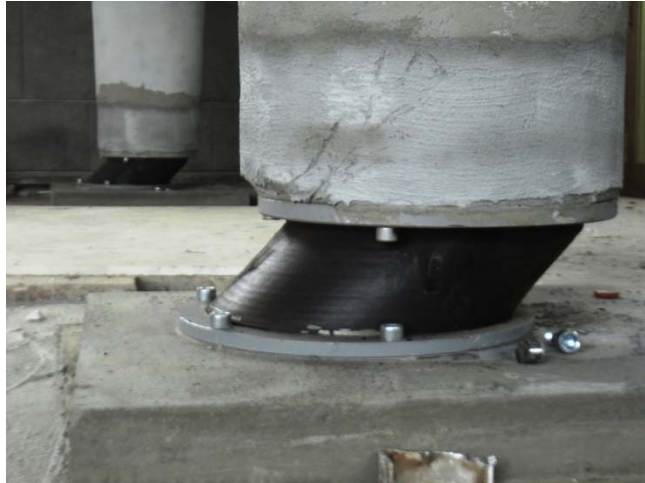
Figure 14. Two of the elastomeric isolators in the deformed configuration, before return to the vertical position.
