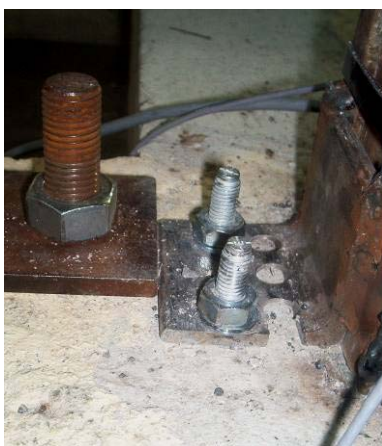
Fig. 11. Damage occurred in the dissipating elements of the 1 st level column at a) top and b) base
