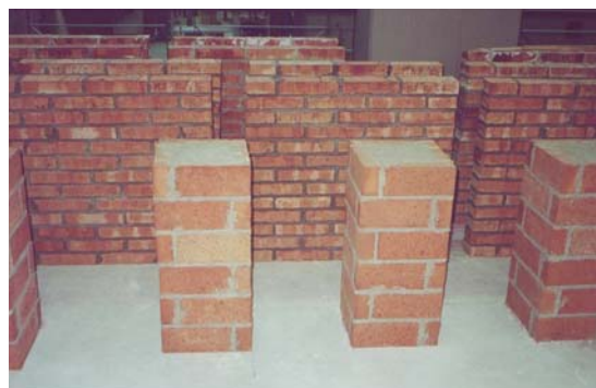
Fig. 13 – Panels and columns before testing.
