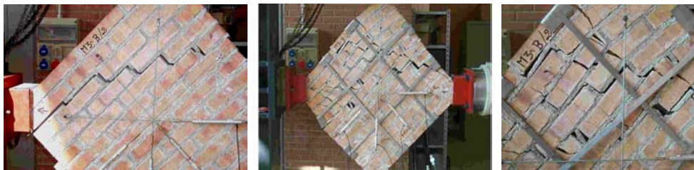
Fig. 17 - a) Failure of the unstrengthened panel b,c) failure of the same panel repaired and strengthened with the CAM System.
