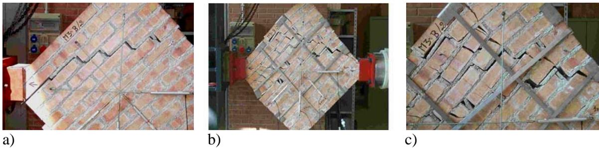
Fig. 14 - a) Failure of the unstrengthened panel b,c) failure of the same panel repaired and strengthened with the CAM System.
