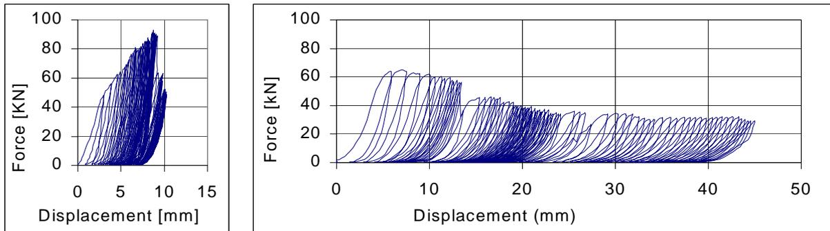
Fig. 16. Diagonal force-displacement diagram of panel M3B1 with CAM strengthening in the third and fourth series of cycles.
