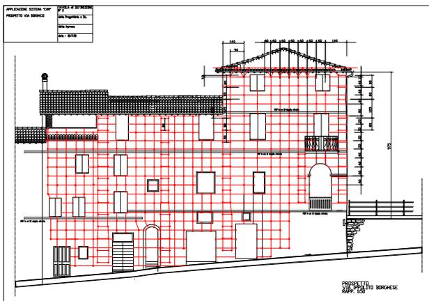
Fig. 8 - CAM arrangement in the facade.
