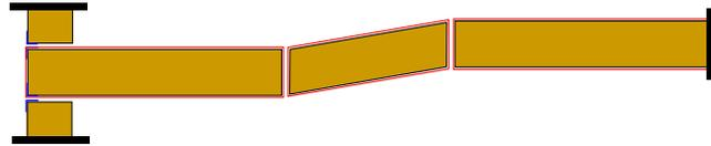
Fig. 7 – Plan arrangement of a tie realised with CAM, which follows the irregularity of the wall.
