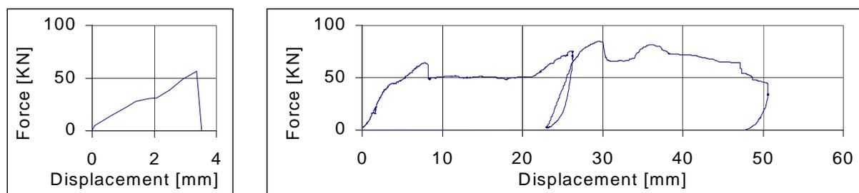
Fig. 15 - Diagonal force-displacement diagram of panel M3B2 without and with CAM strengthening.
